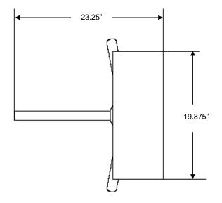
Note: Allow a 2" clearance gap between the end of the turnstile arm and the next unit or outside barrier.
