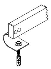
*Product Description:* The CB Cart Bumper is designed to provide case and wall protection.
