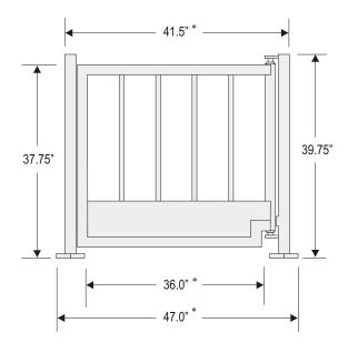
\* NOTE: Dimensions may vary slightly depending on locking mechanism used.
