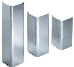
Constructed from 12-guage, heavy duty chrome plated steel, the CPI is installed using four 4 anchors. (Rated at 4,500 lbs. Pullout capacity). Standard heights are 12, 16 and 24 inches. This case protector comes with inside anchors tabs. The CPI is also available in satin finish stainless steel.
