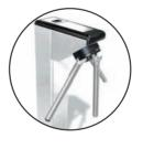
Through an anti-panic mechanism the arm drops leaving the access free. This special feature can be used in emergency cases (activated through a push-button or system in a control room) or in case of power failure (when the turstile does not have the no-break system). The turnstile can also inform the system when the arm drops.
